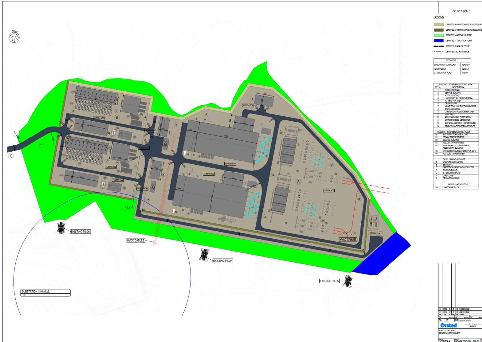
Figure 4: Indicative HVDC OnSS and EBI Layout.
